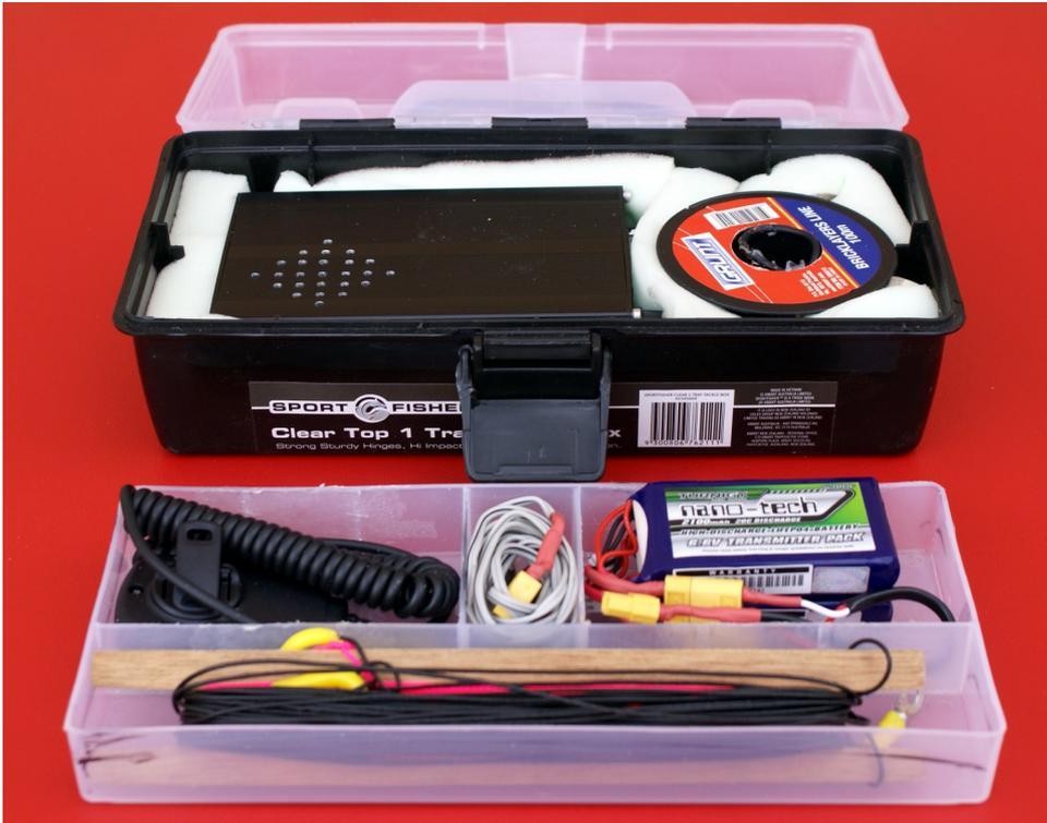
**Above: The packed lunch box. The X1M is at the left in the body of the box and the coax feeder on a spool on the right. The microphone, leads, battery and antenna on a winder all fit in the tray. Note the protective foam used for protection of the rig.**
