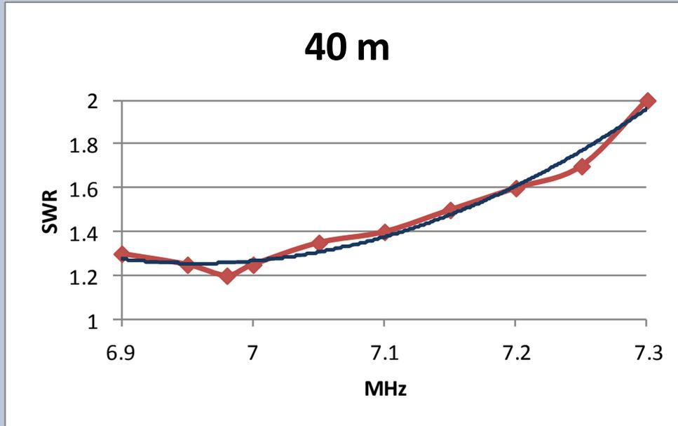
**Fig 4. Measured SWR curve for 40 m.**
