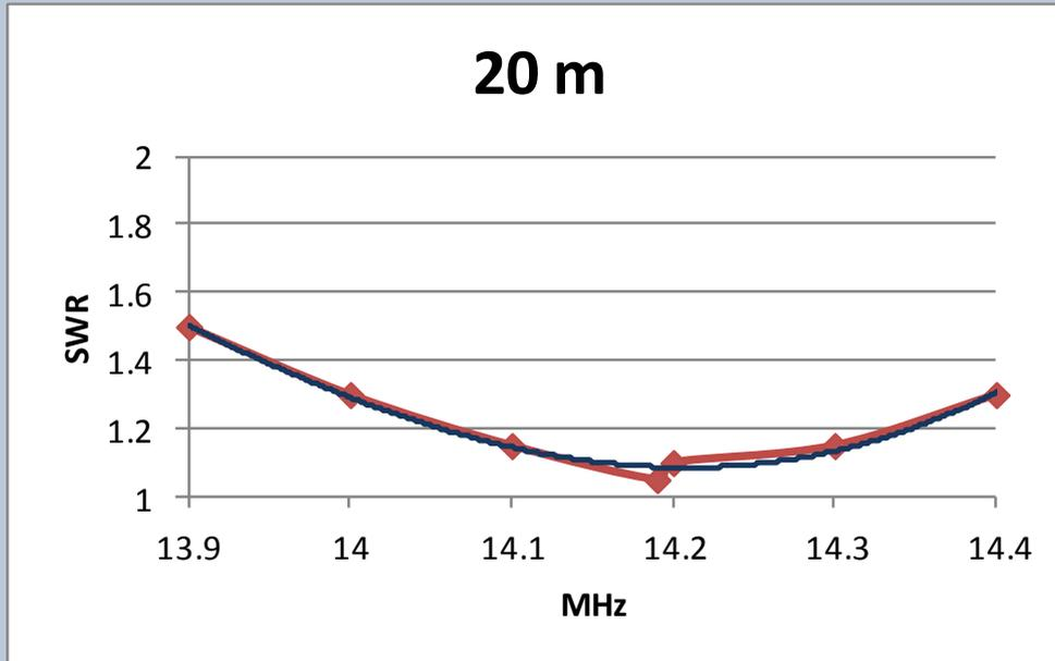
**Fig 5. Measured SWR curve for 20 m.**
