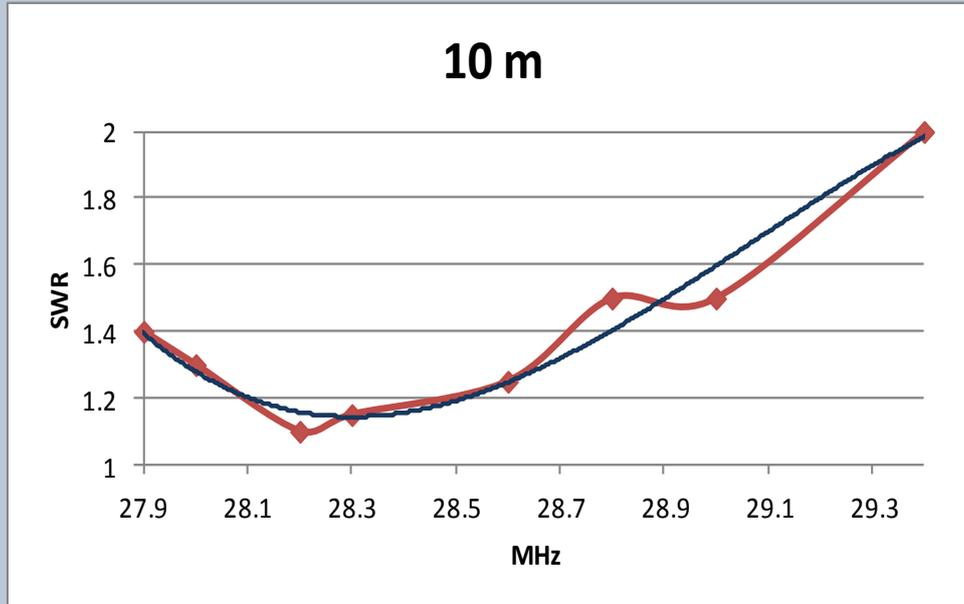
**Fig 6. Measured SWR curve for 10 m.**
