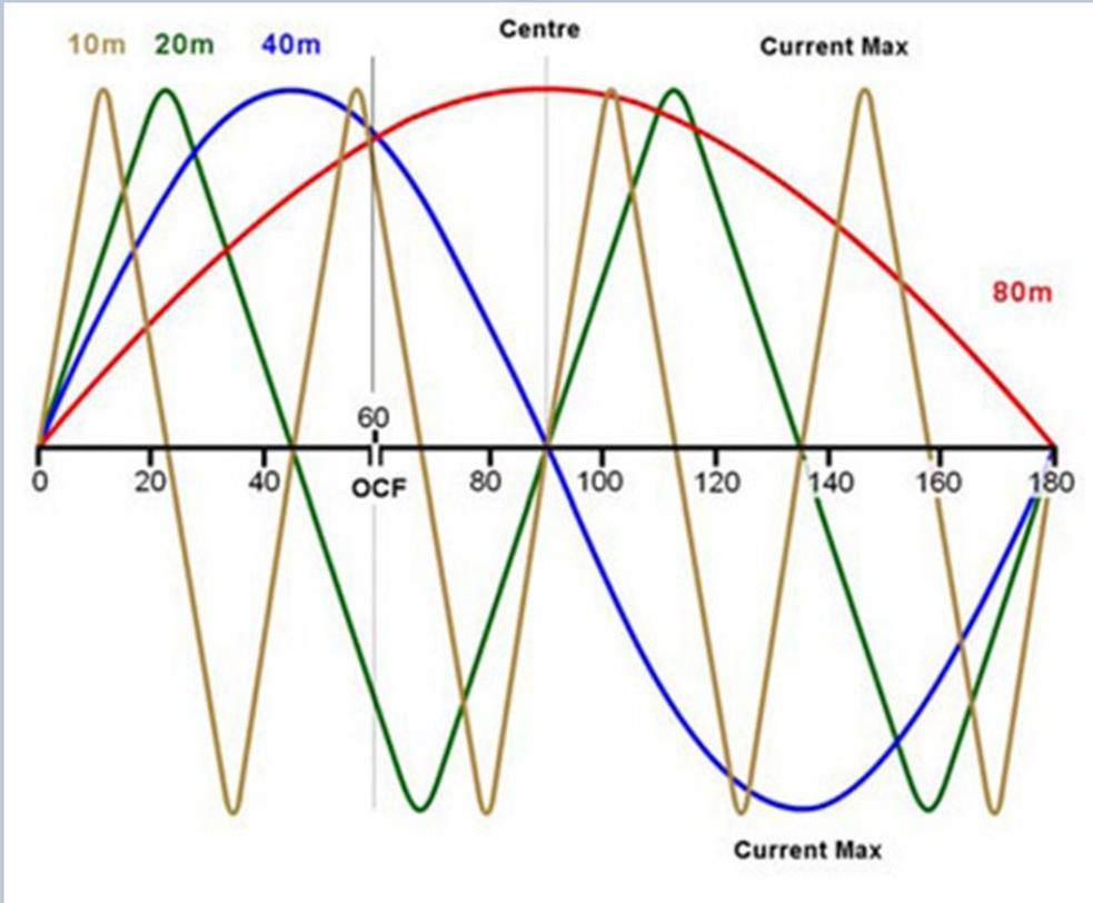
**Fig 1. The fundamental and even harmonic current amplitudes on a 80 m half wave dipole.**
