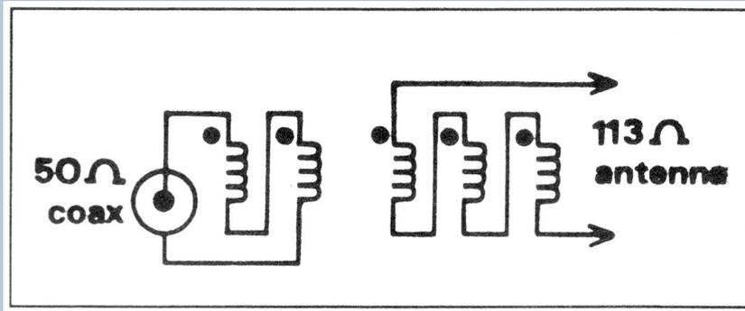
**Fig 2. Balun Transformer wiring**
